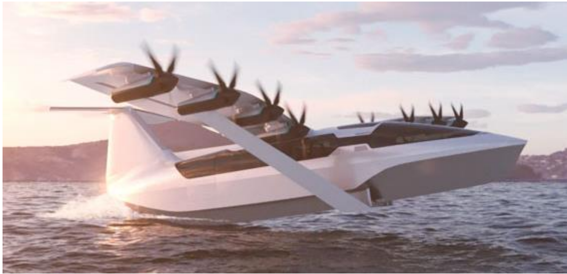
Figure 37. Viceroy electric ekranoplane for 12 pax and 300 km range [Regent]
