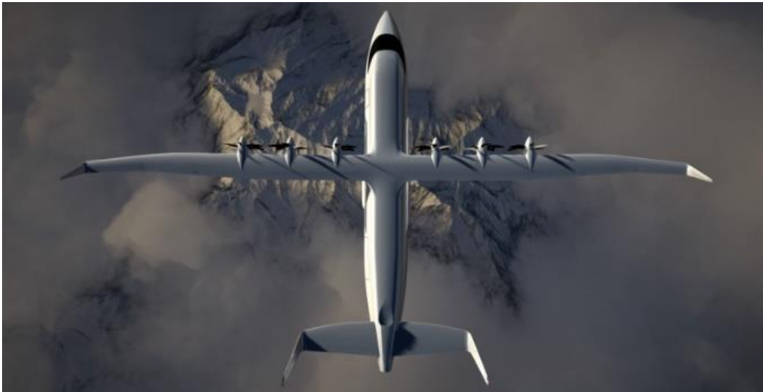
Figure 29. Hybrid model in series of 19 pax. ERA [Aura Aero]
