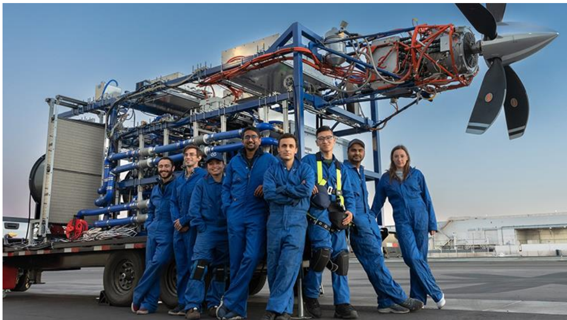
Figure 49. Ground tests of an electric thruster with H 2 batteries of 1 MW power [Universal Hydrogen]
