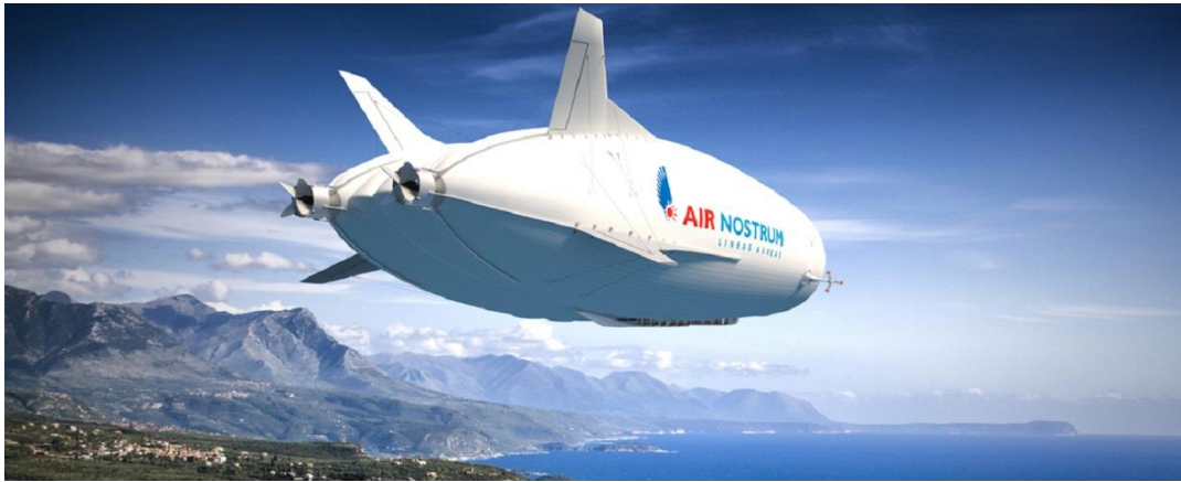
Figure 5. Airlander airship for the transport of up to 100 passengers [Air Nostrum]
