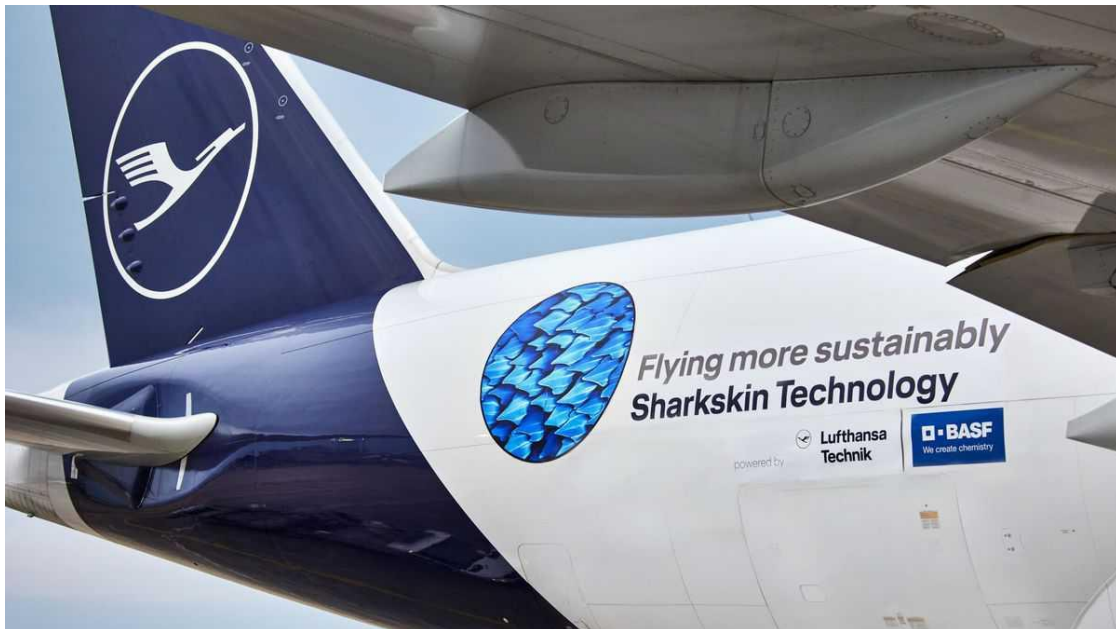
Figure 13. Commercial aircraft with AeroShark surface treatment [Lufthansa]
