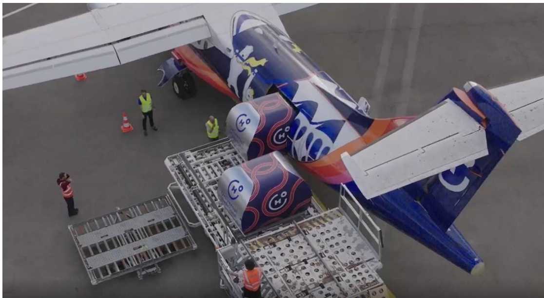
Figure 47. Refueling test using hydrogen containers [Universal Hydrogen]
