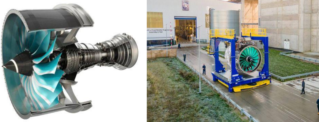
Figure 10. Ultrafan large bypass ratio motor [Rolls-Royce]
