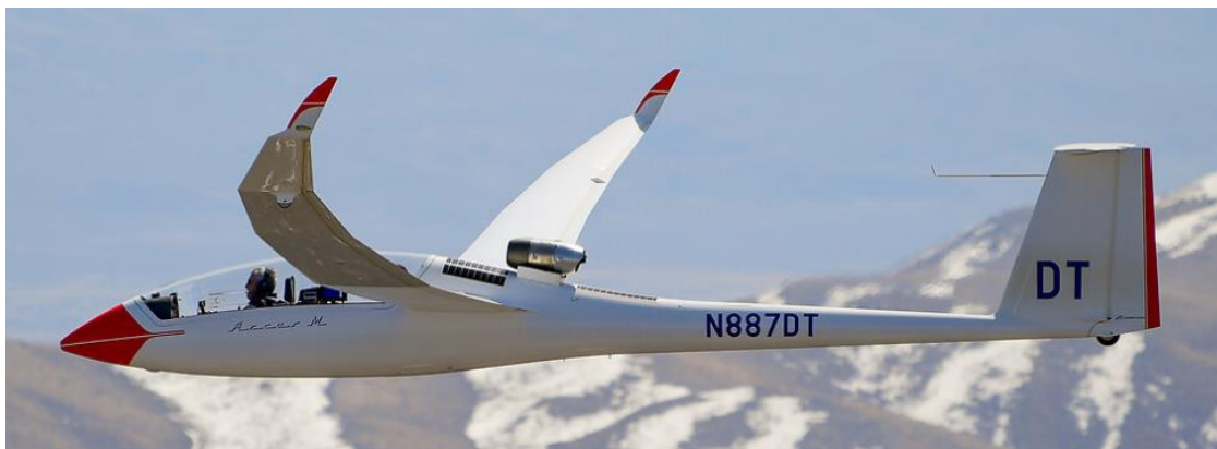
Figure 42. Project Blue Condor glider, fitted with jet engine [Airbus]
