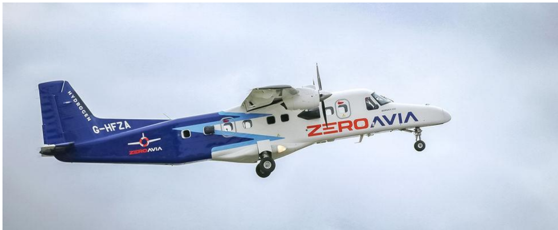
Figure 45. First flight of the Dornier 228 with an electric motor powered by H2 cells [ZeroAvia]
