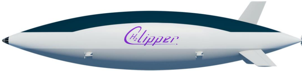
Figure 43. Airship project for the transport of H 2 [H 2 Clipper]
